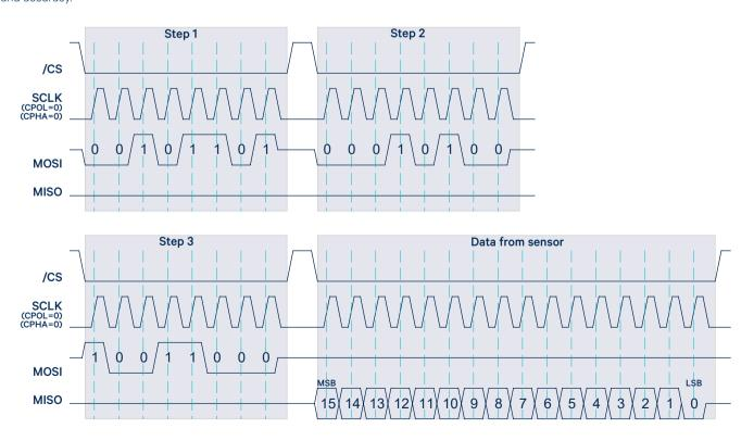
Fig. 5: SPI data transfer
