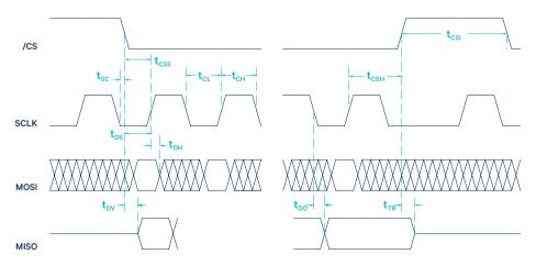
Fig. 6: SPI timing diagram
