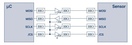
Fig. 4: Application circuit with additional buffer
