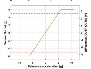
Figure 21: SI1005 versus reference sensor
