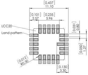
Figure 24: LCC20 land pattern recommendation (units are mm/[inch])
