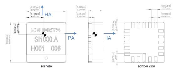
Figure 22: Package mechanical dimension. Units are mm [inch]
