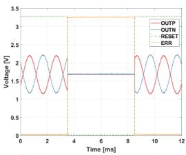
Figure 16: Typical sensor reset sequence with external reset
