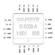
Figure 13: Pinout top view
