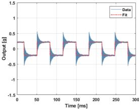
Figure 17: Built-in Self-Test signal on the differential acceleration output (f≈19Hz; a≈±0.25g)
