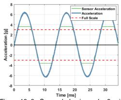
Figure 18: 3g Sensor behavior under 6g sine
