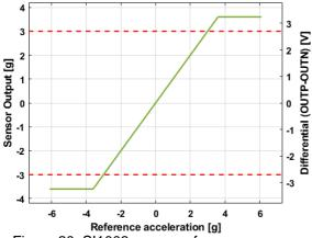
Figure 20: SI1003 versus reference sensor
