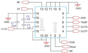
Figure 14: Proximity circuit & internal pull-up/down
