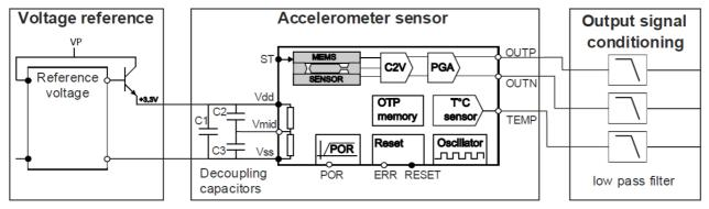
Figure 23: Recommended Block diagram
