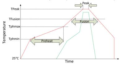
Figure 25: Soldering Temperature Profile
