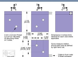
Two 3 mm x 0.5 mm threaded holes are provided on each of three orthogonal faces for mounting
