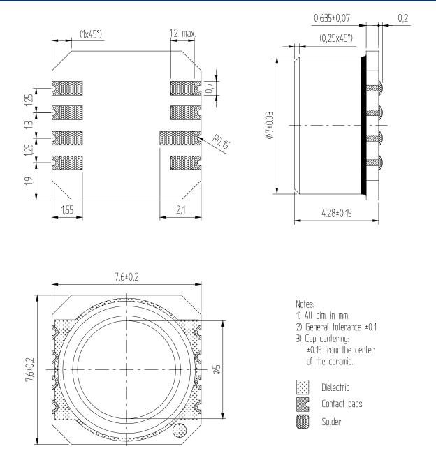
Device package outlines of **MS5212-HM** (Stainless steel cap, with or without gel protection of bonding wires)
