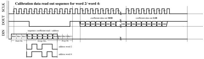
Fig. 6d: W2, W4 READING sequence
