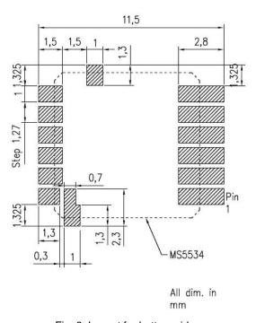
Fig. 9: Layout for bottom side
