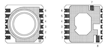
Fig. 2: Pin configuration of MS5535-30C
