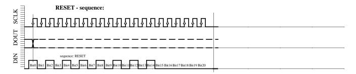
Fig. 6e: RESET sequence (21 bit)
