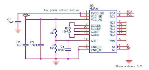
Figure 4: Typical circuit with two-wire interface
