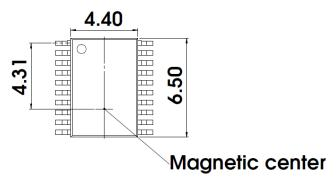
Figure 7: Package drawing (Magnetic center)
