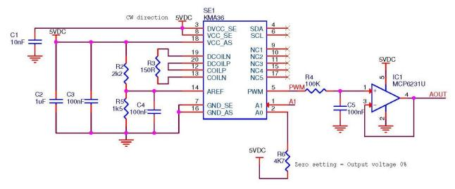
Figure 5: Typical circuit with analog interface
