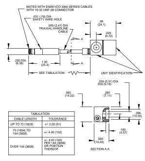
STANDARD TOLERANCE INCHES (MILLIMETERS) .XX = +/- .02 (.X = +/- .5) .XXX = +/- .010 (.XX = +/- .25)
