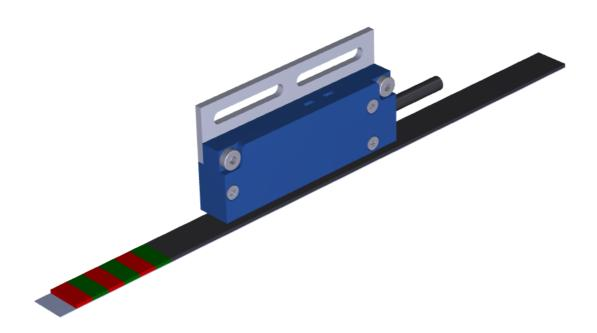
After power on, both LEDs (red and green) should be on. When the red LED goes off, the encoder is in measurement mode. Every millimeter the green LED toggles to give a visual feedback of the measurement. The red LED depicts a missing magnet function, which means the scale is too far away from the encoder or wrong mounted.
